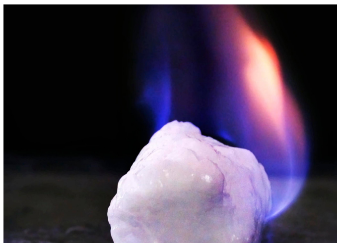
One cubic meter of methane hydrate can produce roughly 160 cubic meters of methane gas, which in turn can be transformed into hydrogen. (U.S. Department of Energy)
