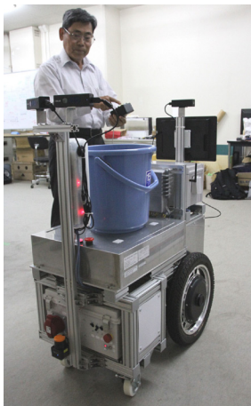
A self-driving, handcart-type robot, being developed to support farmers who grow flowers, is seen at Toyohashi University of Technology in Toyohashi, Aichi Prefecture. | CHUNICHI SHIMBUN
